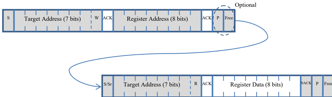
Fig. 9. I2C Control Register Read Sequence Transfer Directions
