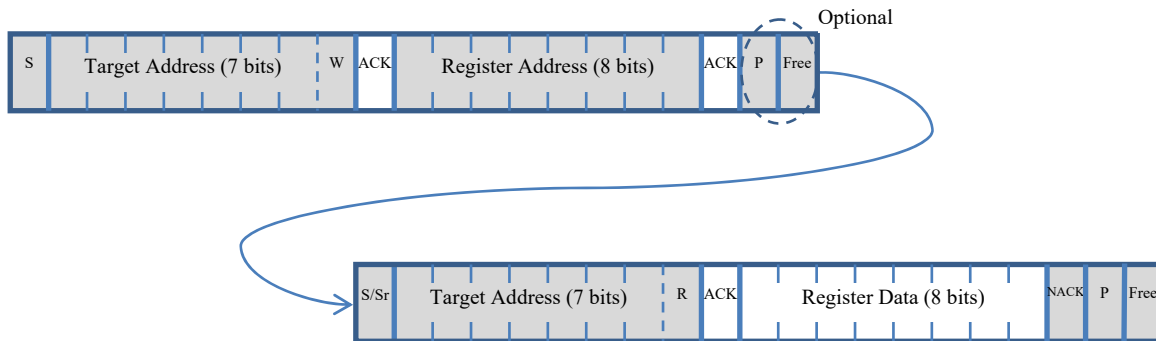
Fig. 9. I2C Control Register Read Sequence Transfer Directions
