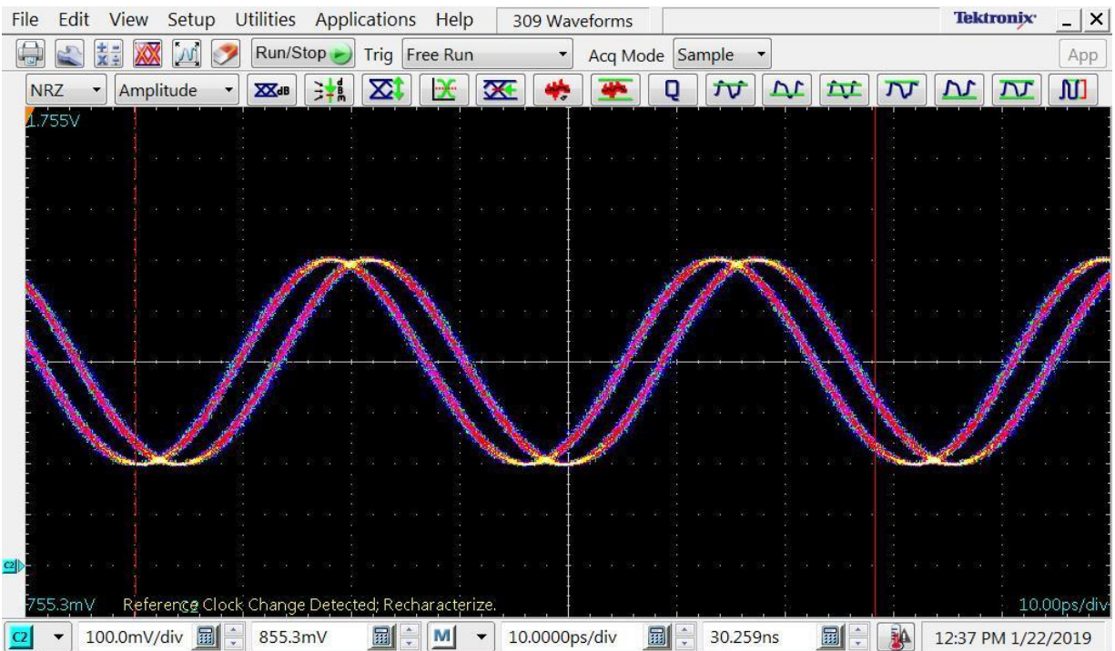
Fig. 4. 28GHz Clock Output of the ASNT9001-JI with inserted internally generated Flicker Noise
